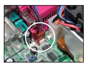
Repeat steps 1 to 2 to install the heatsink and fan assembly for the second CPU, then connect the fan cable to the fan connector labeled CPUFAN2.
